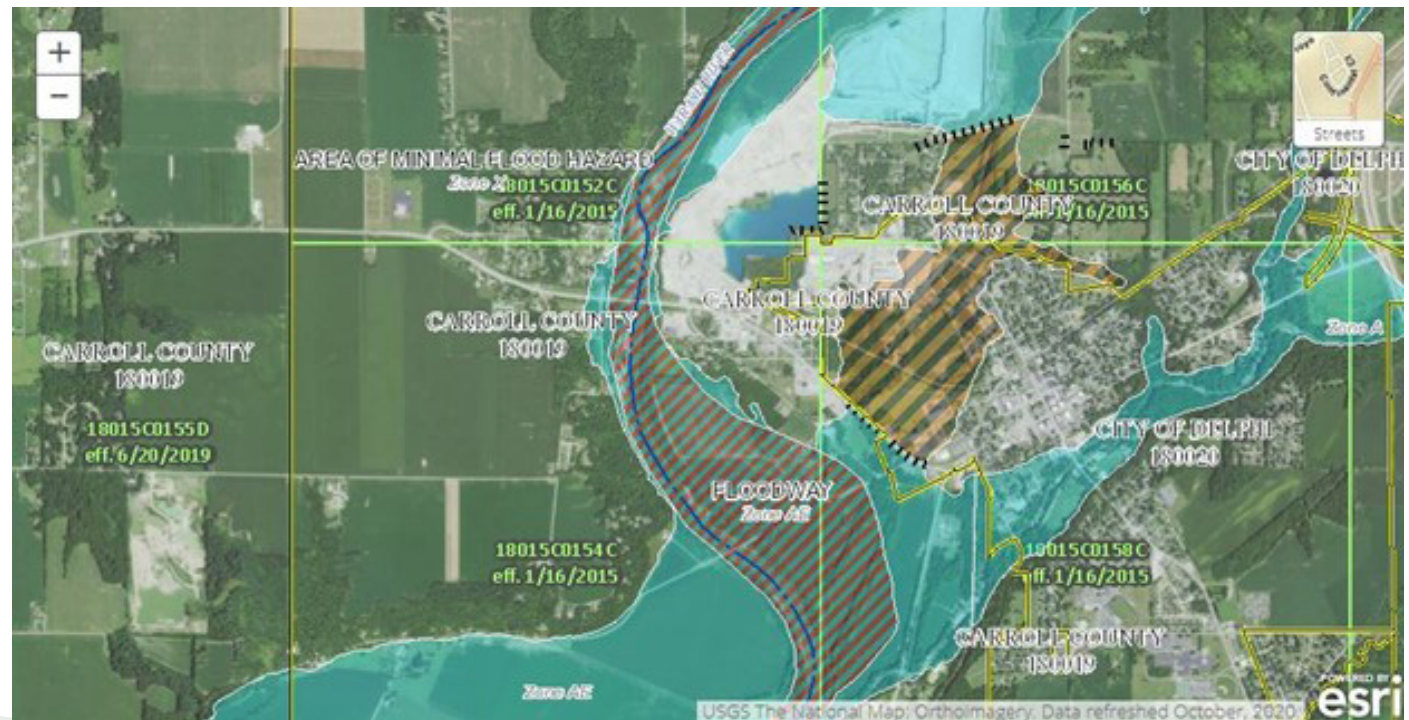
FEMA ZONE AE with Floodway and Zone X also shown (typical for urban areas).
